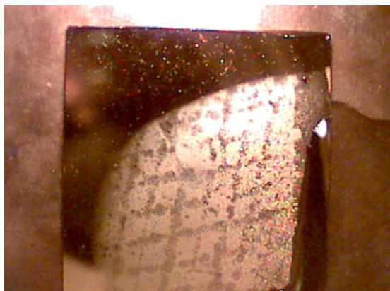
Fig. 2. Condensation of water vapour on a gold substrate spin-coated with an amylose film after an exposure of 8000 \mu\text{C} (2000 \mu\text{C}/\text{cm}^2 ) to electrons with incident energy of 15 eV. The substrate was partially covered by a metal grid during irradiation.
